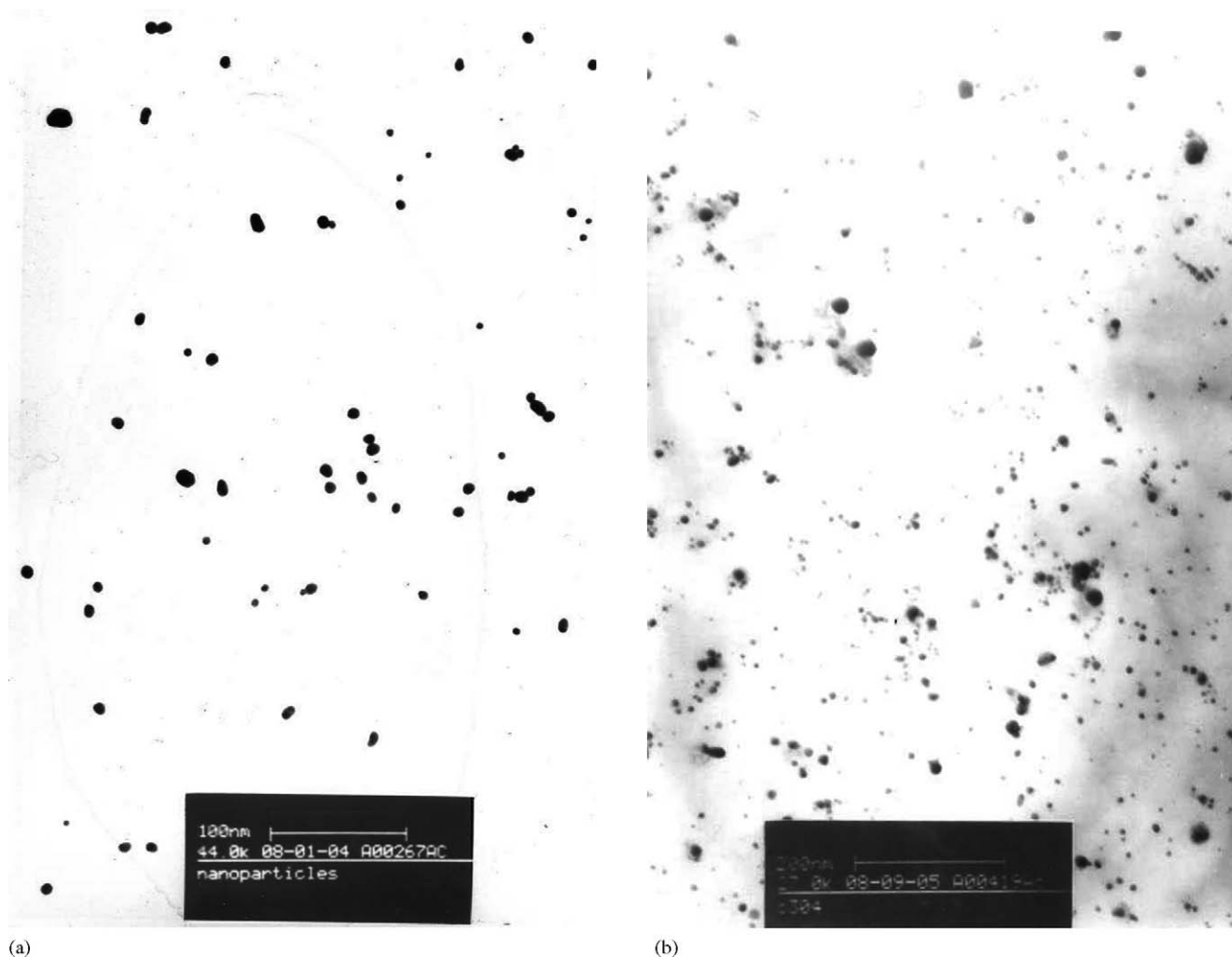
Fig. 2. Transmission electron microscopic images of citrate stabilized metallic nanoparticles: (a) platinum and (b) Pt/Pd bimetallic.
